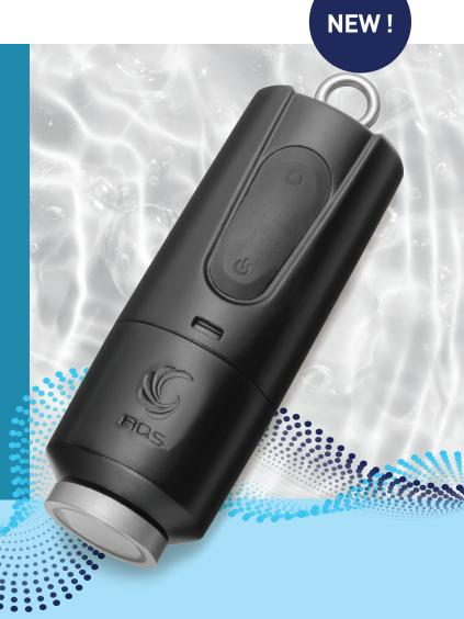
A Piezo based wireless audio recorder (single channel) replacing the legacy iQ100 product. Intended for quick and simple leak survey. Robust design that fits both onto an M8 thread of the listening stick and an attachment magnet. Connecting to the AQS cloud with any mobile phone platform (Android / iOS).
